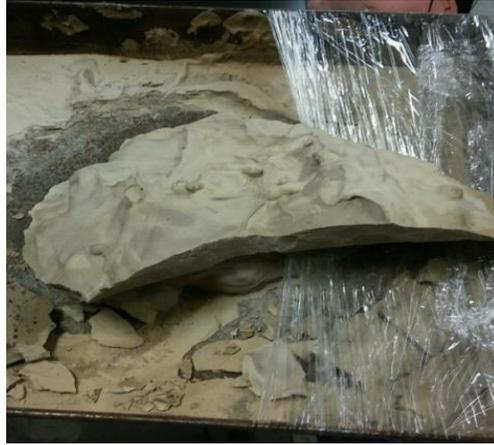
Fig. 2-1. Cementation of class C fly ash sample during mellowing for compaction characteristic test.
