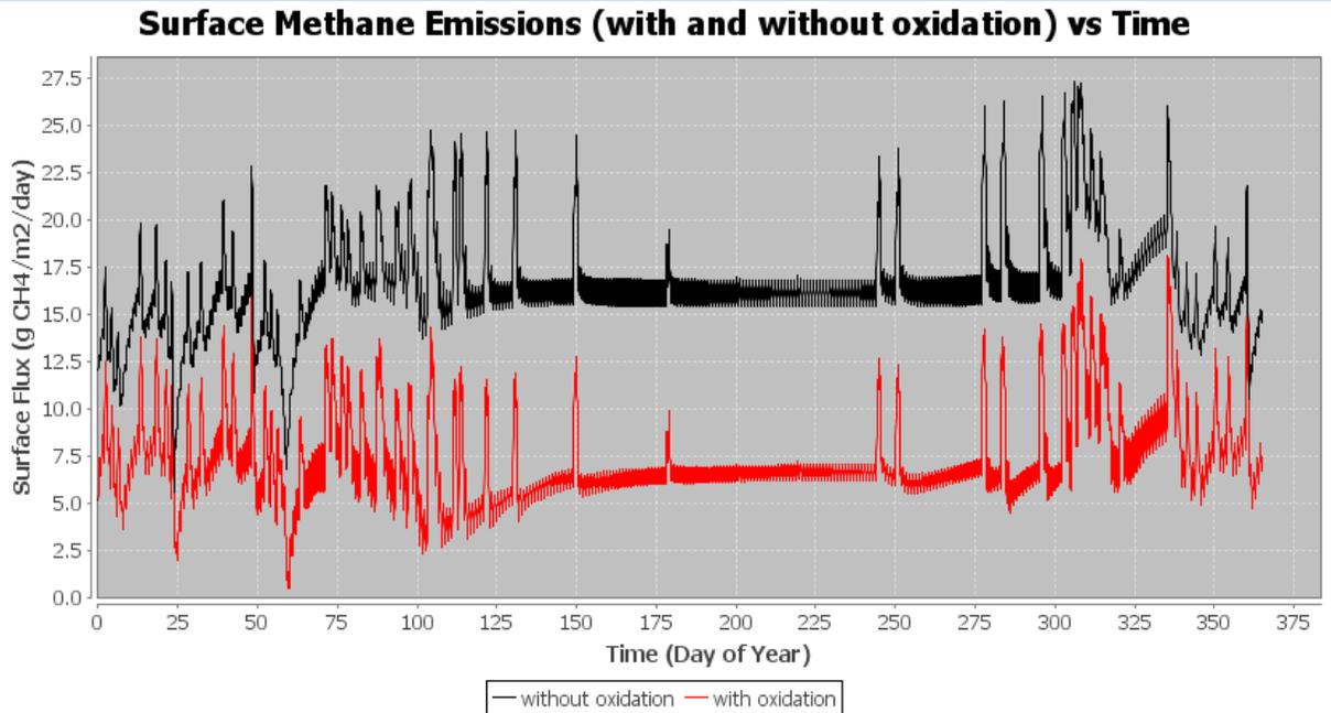
This graph displays the variable surface emissions (10-min. time steps) for a typical annual cycle (365 days) both without methanotrophic methane oxidation (black line) and with methane oxidation (red line) included in the calculations. CALMIM calculates these separately so that the effect of oxidation (difference between the two plots) can be readily seen on this graph.
