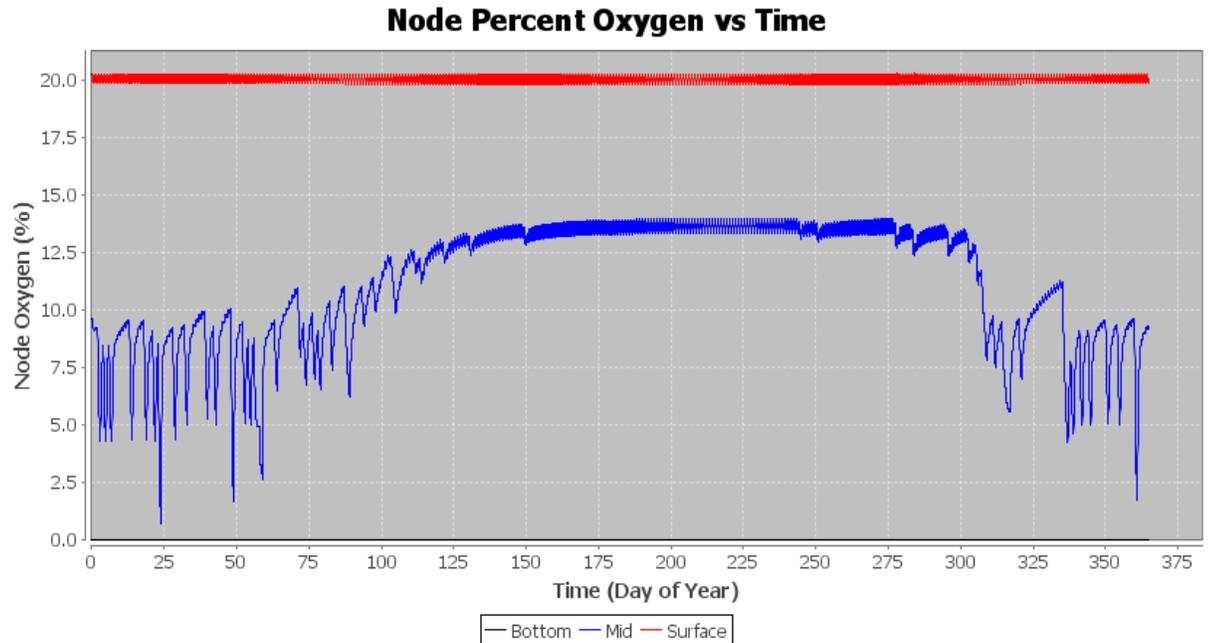
This graph illustrates the surface, mid and bottom node results for soil gas oxygen concentrations (V%) at these 3 respective depths for the selected cover. This value is an indication of the aeration status of the cover soil.
