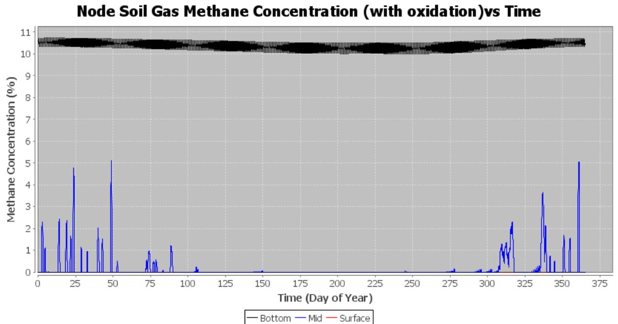
This graph illustrates the surface, mid and bottom node results for soil gas methane concentration (V%) with methane oxidation at these 3 respective depths for the selected cover. methane concentrations with methane oxidation. Note the drastic difference in methane concentrations between the “with” and “without” methane oxidation scenarios. Also note the highly variable methane concentration in the middle layer of this particular cover.
