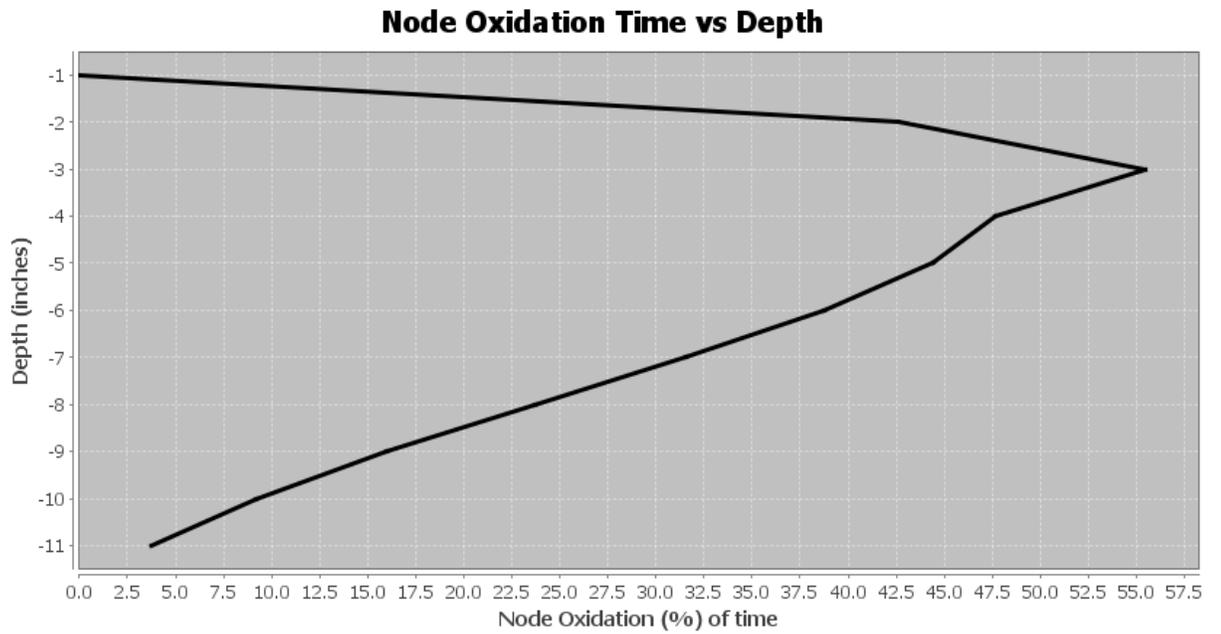
This graph illustrates the percentage of time (over an annual cycle) that each node over the total depth of a selected cover is capable of oxidizing methane.
