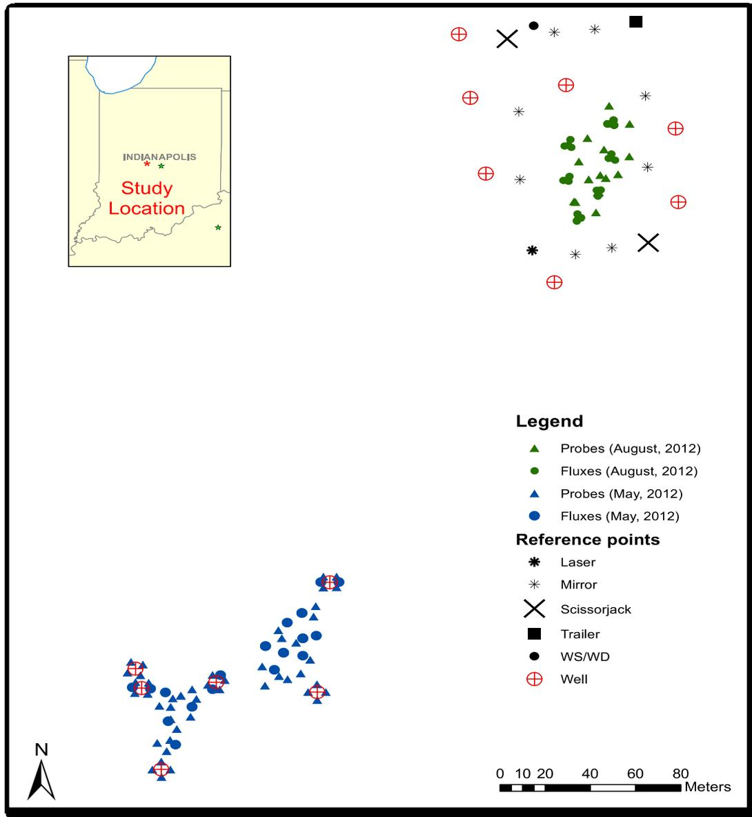
Figure 42. Overview of field monitoring locations at Indiana site IN-1, including locations for soil gas probes, static chamber fluxes, and associated gas recovery wells and other infrastructure in intermediate cover area (May 2012) and extended daily cover area (August 2012).<sup>5</sup>
