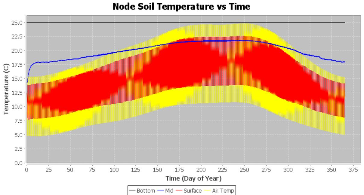
This graph illustrates the surface, mid and bottom node soil temperatures at these 3 respective depths for the selected cover.
