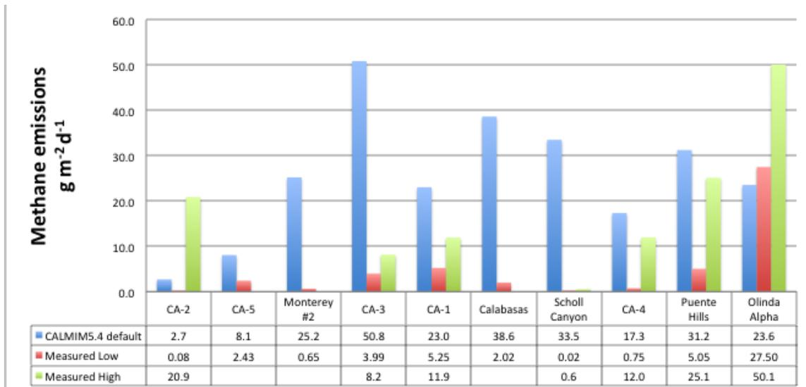
Figure 59. Comparison of modeled to measured CH<sub>4</sub> emissions (various dates 2006-2012; methods include static chambers, VRPM, tracer methods, micrometeorological methods, and aircraft-based mass balance methods). See Appendix B for detailed site information. High results for Olinda-Alpha and Puente Hills are both from Peischl et al., 2013.
