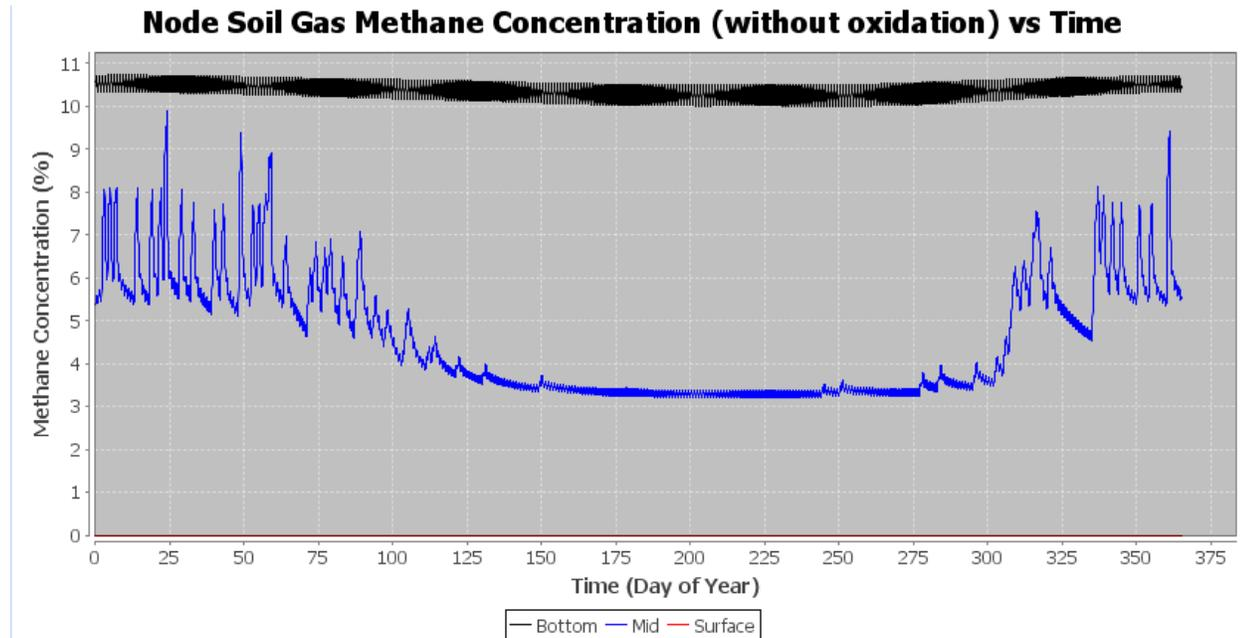
This graph illustrates the surface, mid and bottom node results for soil gas methane concentration (V%) without methane oxidation at these 3 respective depths for the selected cover.
