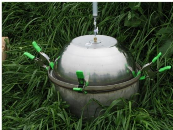
Figure 9. Photo of stainless steel flux chamber used for Indiana Field Project
