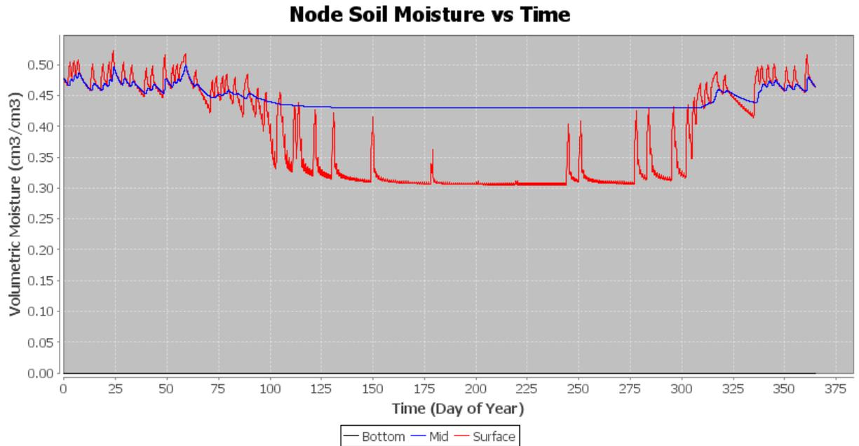
This graph display the surface, mid and bottom node results for volumetric soil moisture at these 3 respective depths for the selected cover.
