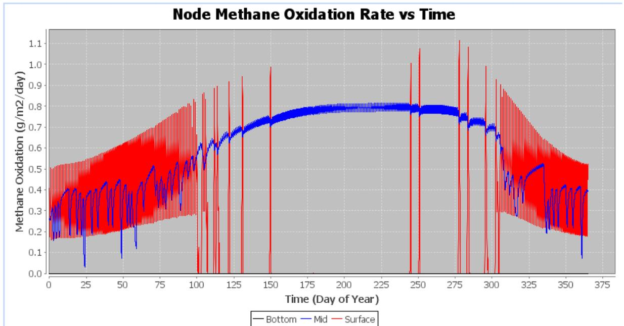
This graph illustrates the total methane oxidation rate per node (in units of  $\text{g CH}_4 \text{ m}^{-2} \text{ day}^{-1}$ ) at the same 3 respective depths for the selected cover. Note that this is calculated separately for each node and is NOT the methane surface emissions.
