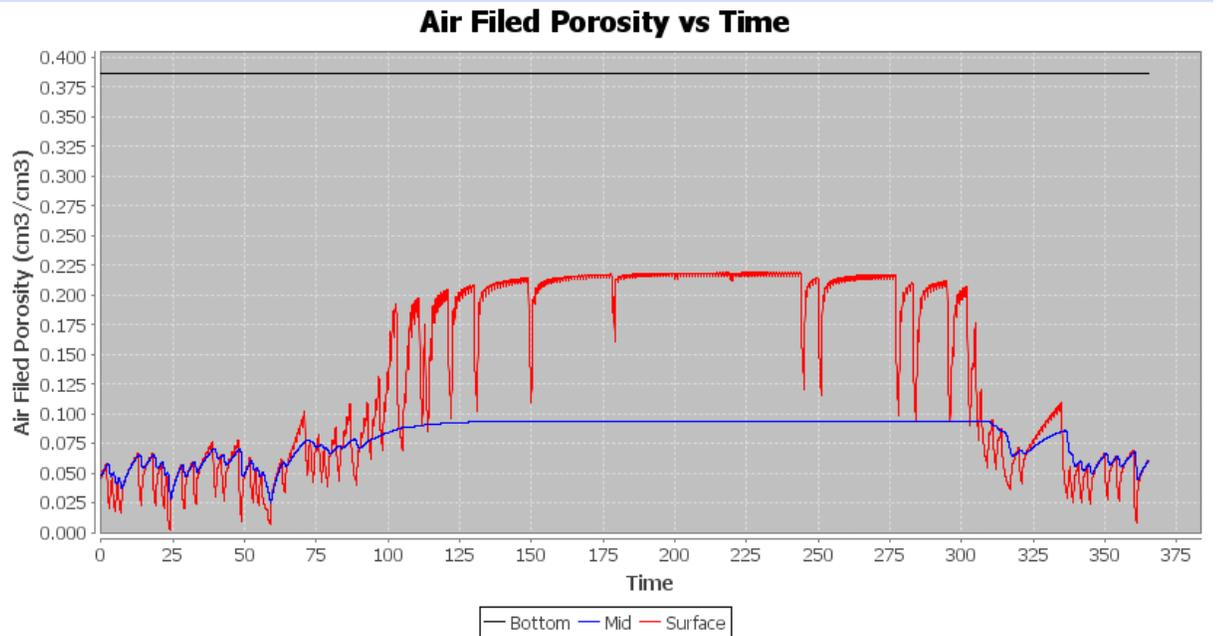
This graph illustrates the surface, mid and bottom node alterations in air-filled porosity at 3 depths for the selected cover. Air-filled porosity changes as a function of the fluctuating soil moisture conditions.
