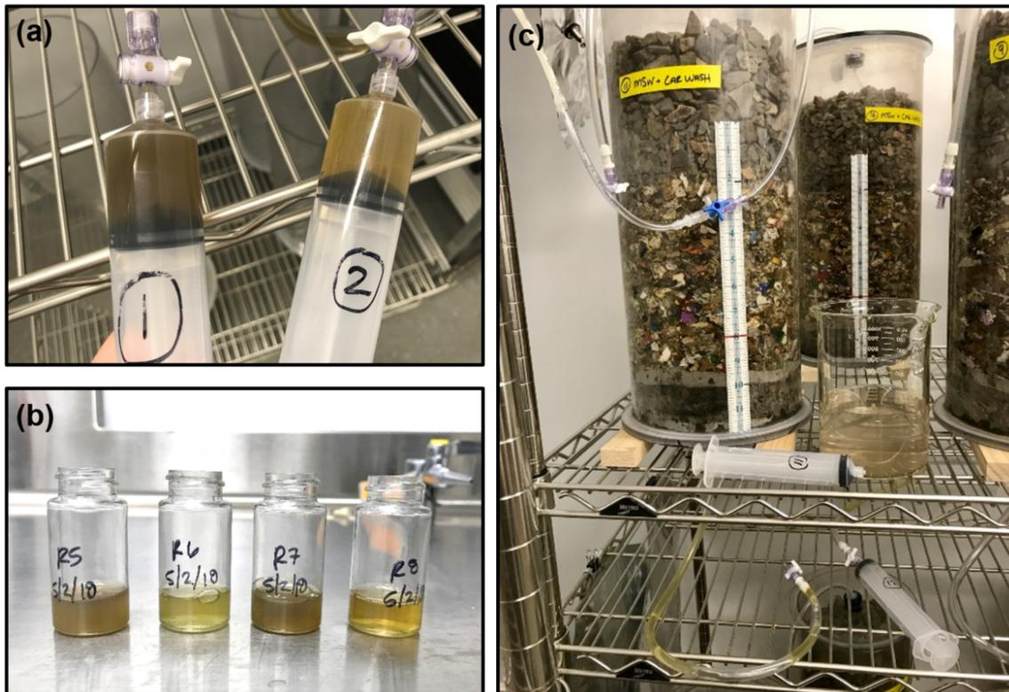
Figure C-3. Weekly recirculation: (a) reactor leachate is pulled from the gravel storage layer via syringe, (b) samples are collected and stored in vials, and (c) leachate volume is measured via syringe, collected in a beaker, and buffered before reinjection into the influent port.
