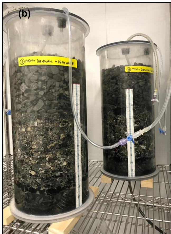
Figure C-6. Operational considerations including (a) reactor clogging due to AD sludge addition and (b) sulfate reduction, indicated by the black coloration in the GB reactors.
