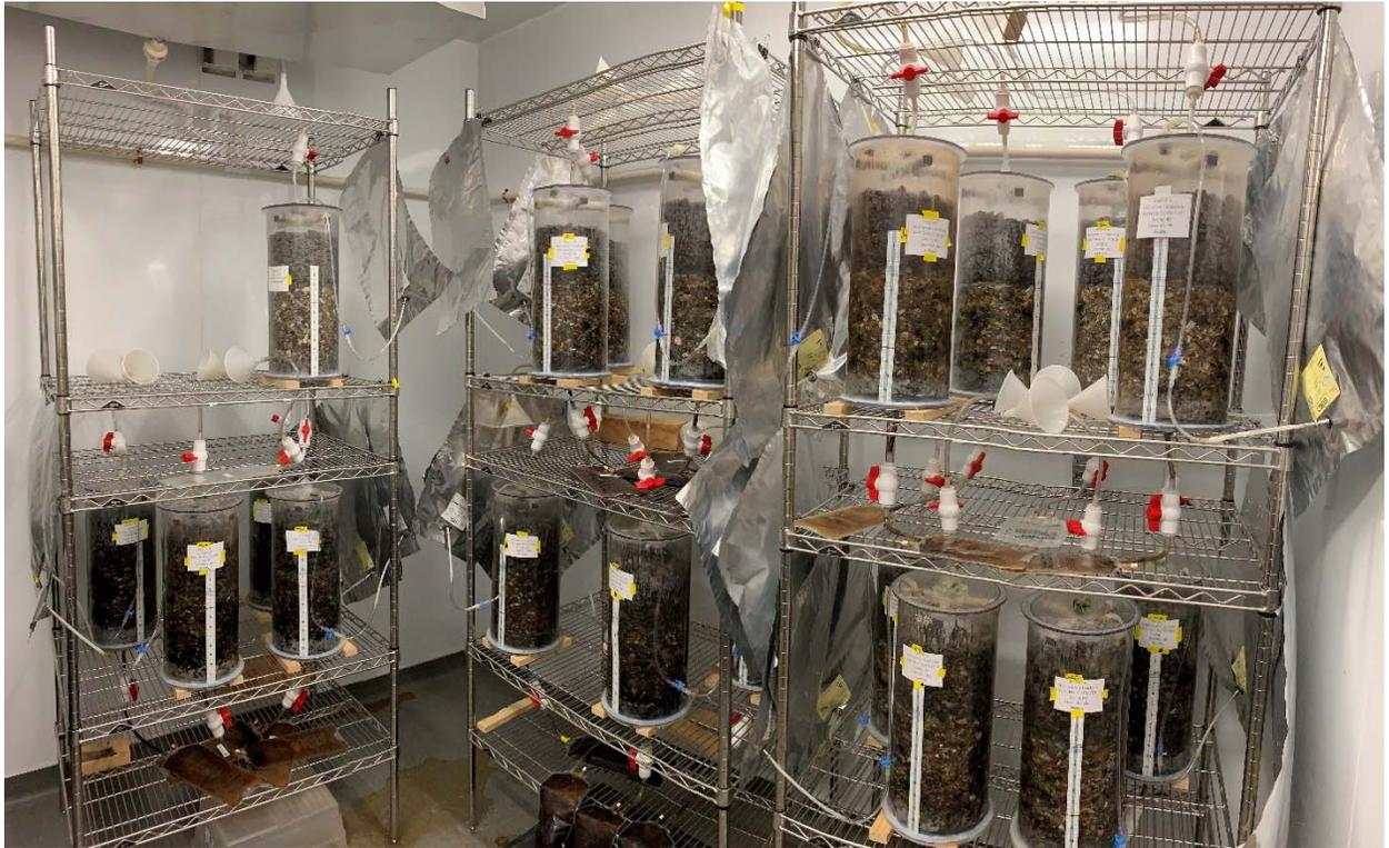
Fig. E-5. Reactors during operation in the temperature control room.
