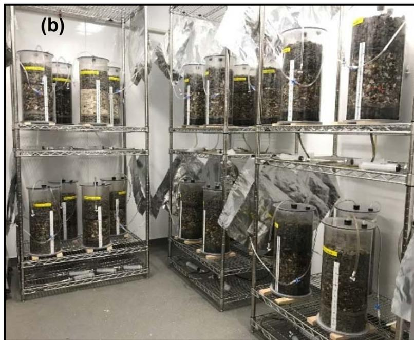
Figure C-2. (a) Final constructed control reactors and (b) temperature control room with 24 reactor experiments in operation.
