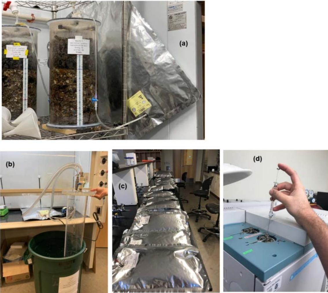
Fig. E-2. Reactor gas management: (a) biogas collection system; (b) biogas measurement apparatus that included a 10-L inverted graduated cylinder, vacuum pump, and acidified water with  $\text{pH} \approx 3$ ; (c) filled gasbags acclimating to laboratory temperature; and (d) injecting biogas sample into GC machine.
