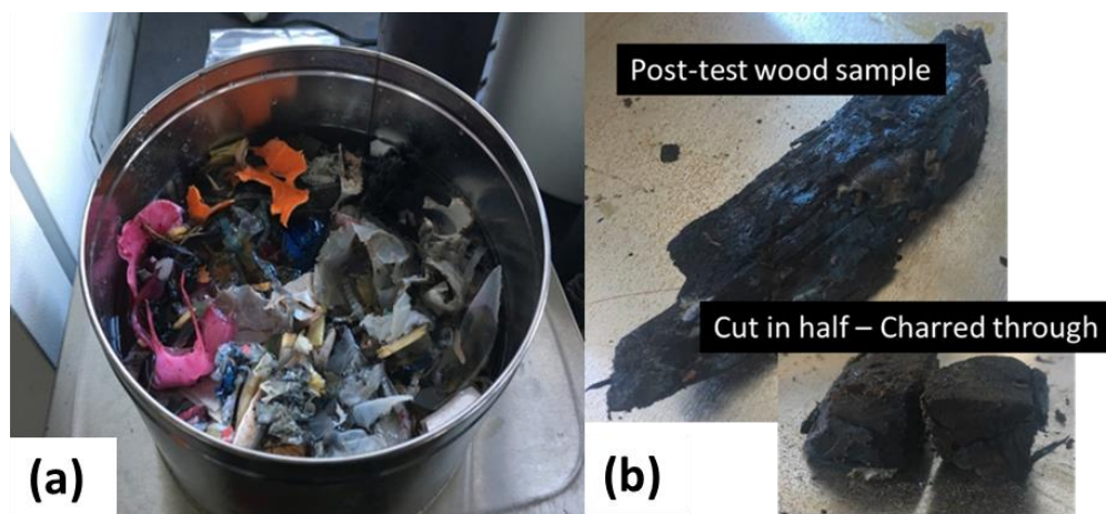
Figure 4-9. (a) Synthetic MSW prior to Phase 1 test and (b) post-test wood sample showing charring
